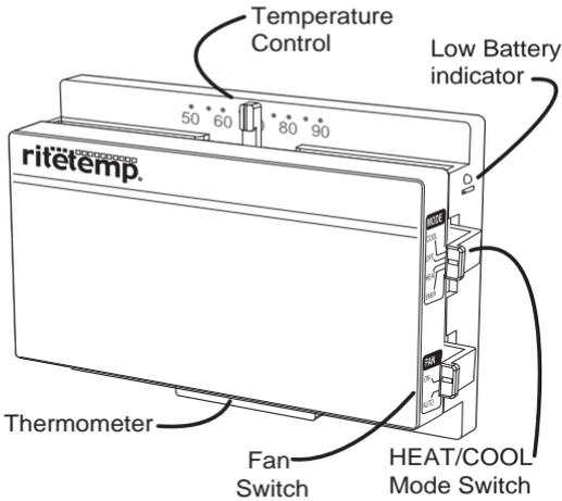
Statement of use: The GPMG8010 can be used with most 24 volt gas, oil or electric heating systems, zoned heating systems, heat pumps with or without auxiliary heat, or gas millivolt heating systems. **It cannot be used with 120 volt heating systems.**
