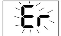
To correct this problem, replace the batteries with 2 new AA alkaline batteries, even if you have recently replaced them. Next, use a paper clip to press the RESET button next to the keypad. You will need to reprogram your thermostat and confirm normal operation.
